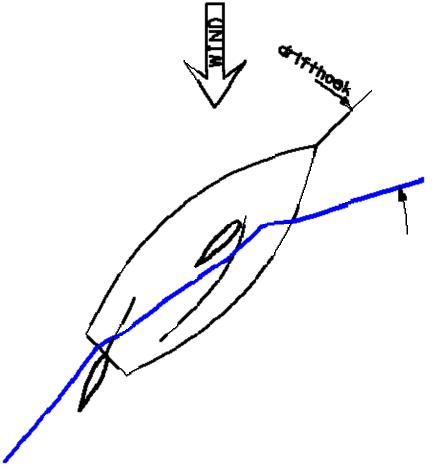
Please note above picture is exaggerated. The right balance can be obtained with moving the sail force by moving or raking the mast, or with the heel.
